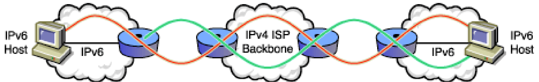
Router-to-Router and Router-to-Host Automatic Tunneling
